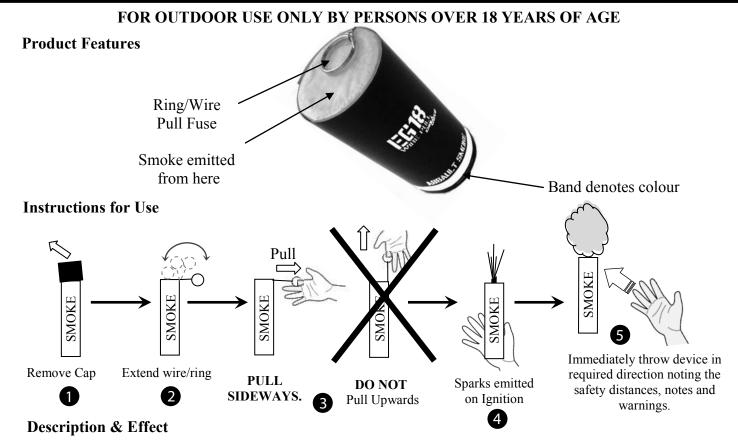
On Ignition there is a 4-5 second delay, the device then produces non toxic smoke for approximately 1 minute. The colour of the smoke produced is denoted by the colour of the band at the bottom of the Label.
